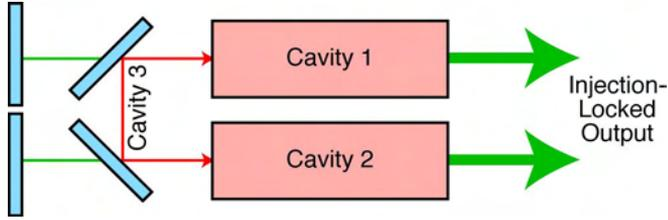
Fig. 5. Mutual injection locking shares portions of the signal from each cavity with the other, resulting in linking three cavities: the two independent oscillators, Cavity 1 and Cavity 2, and the virtual cavity formed by the coupling, Cavity 3.
