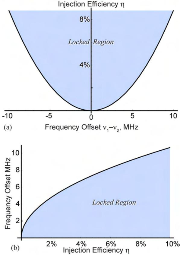
Fig. 3. Relationship between injection efficiency and maximum frequency offset demonstrates that, for a 100-cm perimeter cavity and injection-locked gain of 2, an injection efficiency of nearly 10% is required to lock two cavities, the natural frequencies of which vary by 10 MHz. The frequency offset in this figure is  $\nu = \omega/2\pi$ .
