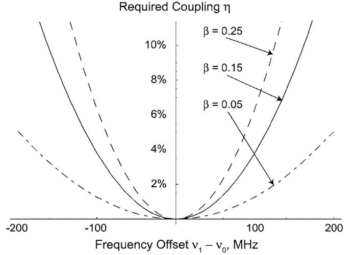
Fig. 6. Level of intracavity coupling required for full mutual injection locking increases with  $\beta$ , the coupling parameter defined in (14).
