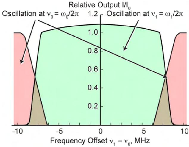
Fig. 4. Relative output of the cavity used as an example in this section shows that, within the locked range of  $\pm 7$  MHz, the system produces greater output at  $\nu_1$  than the free-running laser would at  $\nu_0$ . Outside the locked range, the system acts as a free-running oscillator. There is also a transition range over which both  $\nu_1$  and  $\nu_0$  are produced.
