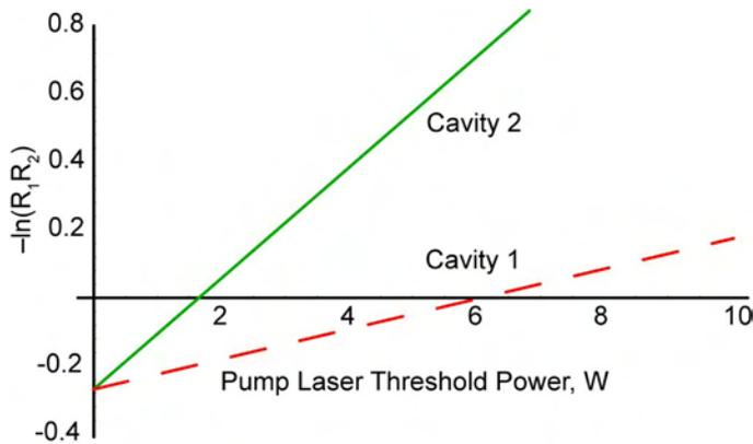
Fig. 8. By plotting oscillation threshold versus mirror reflectivity, one can extrapolate the internal cavity losses and demonstrate the effects of pump size, shown by the different slopes of the two lines.
