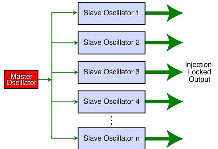
Fig. 1. In a traditional injection locking system, a master oscillator injects part of its output into at least one slave oscillator.
