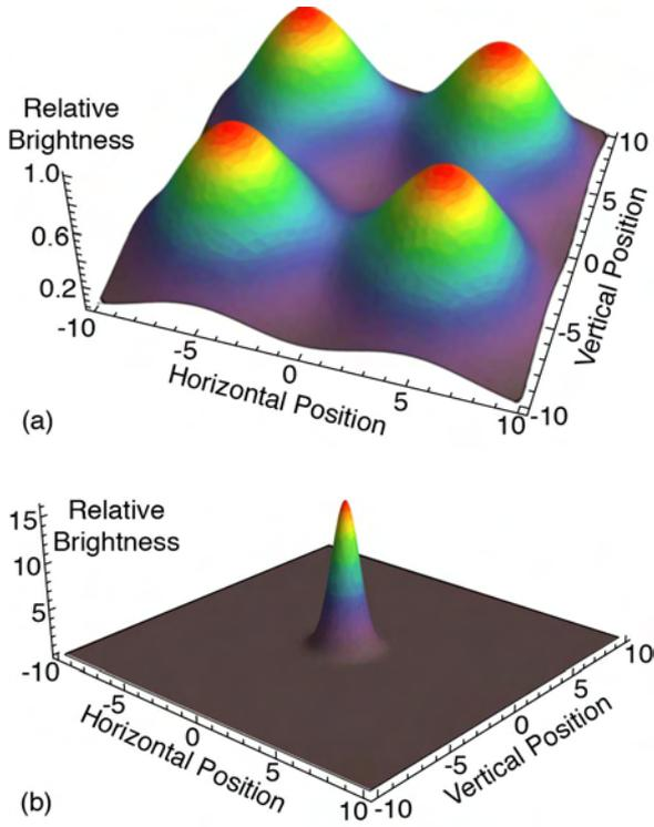
Fig. 2. (a) In the near field, a four-element phase-locked array acts as four independent oscillators, as does an incoherently combined array in the far field. (b) The phase-locked array output, however, combines into a single narrow high-quality beam. All beams were modeled as lowest order Gaussian and propagated with the Fraunhofer propagation equation.
