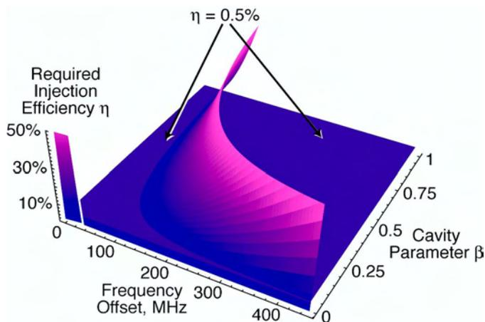
Fig. 10. As cavity parameter and frequency offset increase, the injection efficiency required for mutual injection locking also increases.
