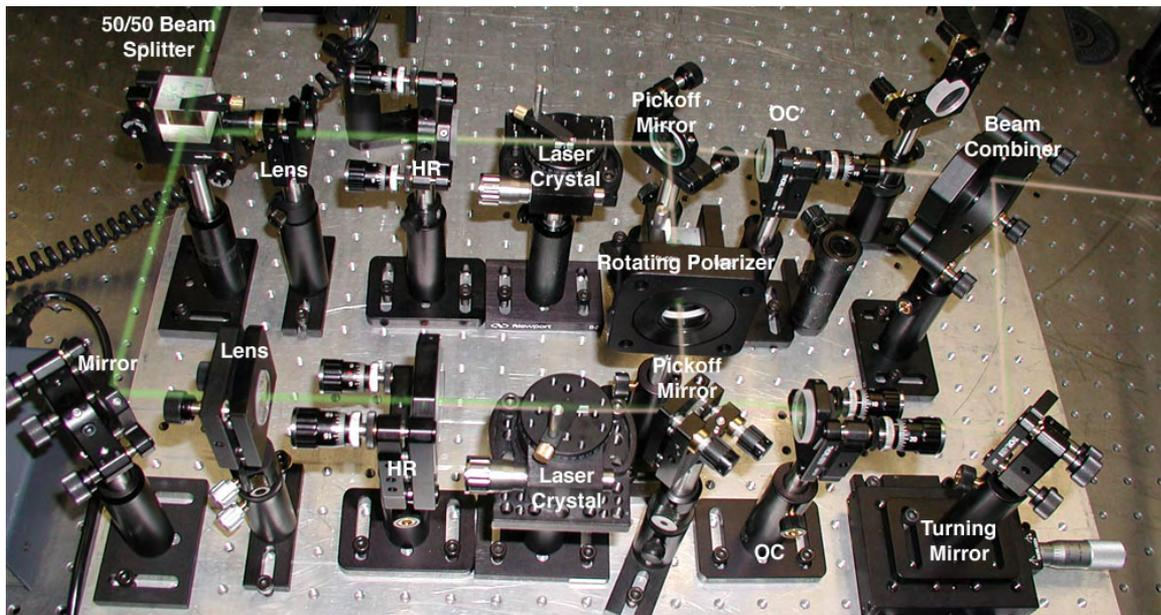
Fig. 7. Mutual injection locking experiment included two independent laser oscillators, coupling within the cavities, and a method of combining the two output beams to measure mutual coherence.
