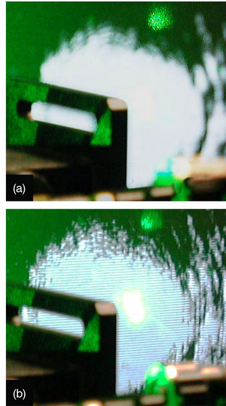
Fig. 11. (a) At mutual injection efficiency 0.4%, even Cavity 1 is oscillating in low-order modes. (b) At 0.5% efficiency, the pattern formed by interference between outputs of the two cavities demonstrates that they are fully locked, operating at the same frequency with only a constant phase difference.
