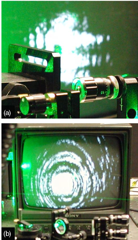
Fig. 9. Beam quality observed from (a) Cavity 1 is significantly lower than that from (b) Cavity 2.
